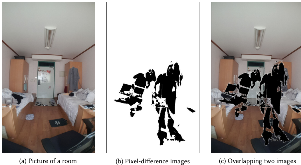
Fig. 3. Inferring movement context from pixel-difference images. Image (b) shows how pixel differences are saved when someone is moving from the bed to the desk, or vice versa.
