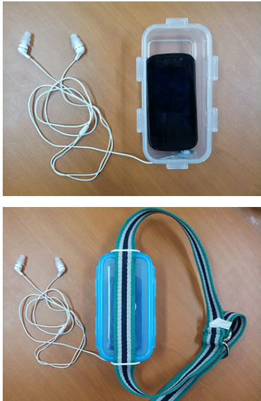
Figure 1. A smartphone in a waterproof housing with an elastic belt; the earphone jack comes out through a hole caulked with silicon.
