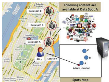
Fig. 1. DataSpotting overview: Black lines represent Alice walking through data spots. The DataSpotting server maintains a data spot map and creates content profiles for each data spot.
