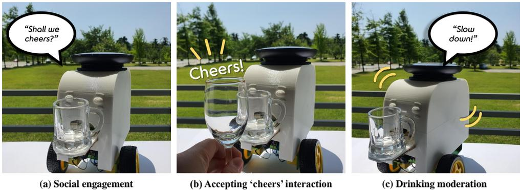
Fig. 1. Three main interactions with the companion robot. (a) Social engagement: The robot suggests clinking to make it more enjoyable, (b) Accepting ‘cheers’ interaction: When the user offers a toast, the robot accepts it and the user can clink the glass with the robot, (c) Drinking moderation: The robot also regulates drinking when the user drinks too fast by talking and shaking its body.
