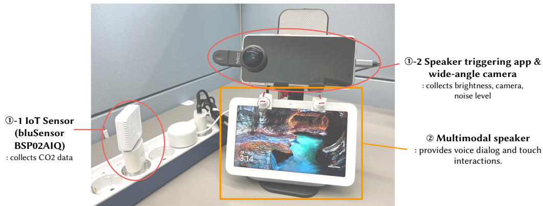
Figure 2: Overall hardware configuration of the system
