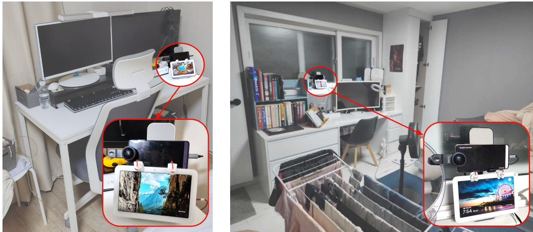
Figure 7: Photos of installed smart speakers: The system was installed in places such as desks and bedsides, where the wide-angle cameras of the mobile phone can scan the entire room and users feel comfortable interacting.
