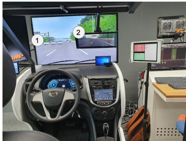
Figure 9. Descriptions of how the participant responds to the emergency braking situation (Source: Own creation): (1) the participants can use the frontal windshield since the telematics system does not support the function that informs frontal situation information and (2) the participant can recognize the rear situation through the rear camera.
