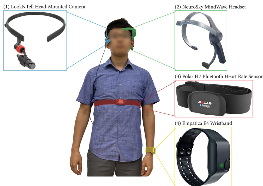
Fig. 2 Frontal view of a participant equipped with wearable sensors.
